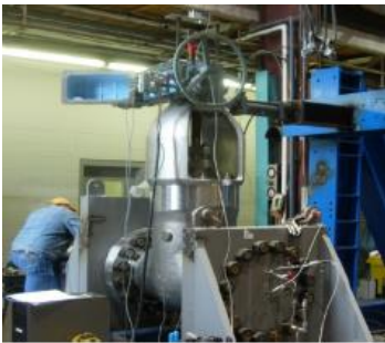
QME-1 TEST for Motor Operated Valve in Nuclear Power Plant
