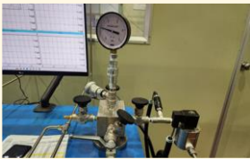
Further control valve Pressure gauge
