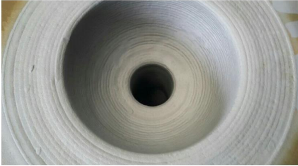
Photo of cladding inside the bonnet of the 20inch-2500# GATE VALVE
