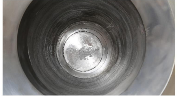
Photo of cladding inside the body of the 20inch-2500# GATE VALVE
